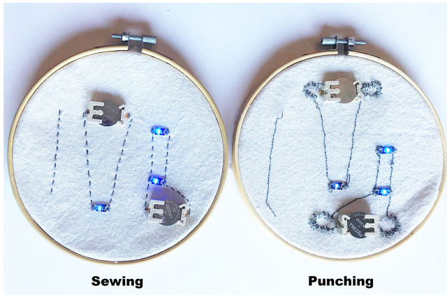
Figure 3: The activity examples participants were shown before starting (left) sewing e-textiles with a sewing needle (right) Punch-Sketching e-textiles with a needle punch tool. It took participants an average of 45.40 minutes to sew their circuits, 11.42 minutes to take apart the sewing whereas punching took on average 28.12 minutes and 1.44 minutes to take apart their punched circuits
