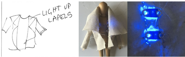
Figure 9: With practice practitioners can use the punch needle to quickly prototype 3D objects in-situ without a tension frame. In this example, a wearable jacket concept goes from sketch (left), to quick mock-up using the punch needle (middle), with a close up of the punched stitches (right)
