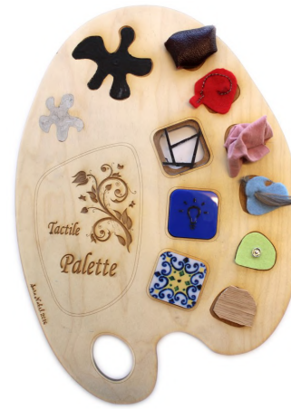
Figure 3. Tactile Palette: a design tool created for Case Study 2 for introducing capacitive-sensing embedded within different interior finishing materials (e.g. wood, fabrics, leather, glass, acrylic, ceramic).
