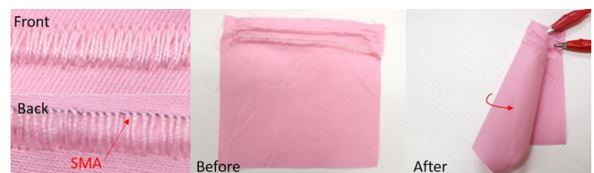
Figure 13. Technique 9: Machine-sewing bobbin-trained SMA wire with thread. After actuation, the fabric rolls around itself.
