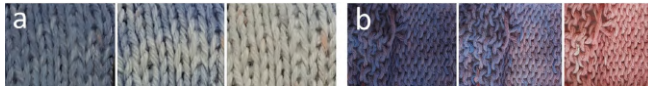
Figure 5. Gradual colour-change of (a) white and (b) pink knitted yarns dyed in blue thermochromic pigments.
